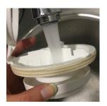
Pull down the bottom section of the NOOD water trap to release the spring-loaded mechanism. Hold the NOOD water trap open in this way while cleaning. You can use an old toothbrush or your finger to clean any dirt from the trap.
